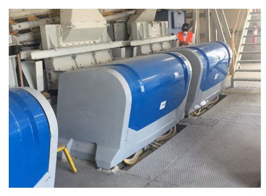
sorting process for the separation of plastic, paper, and metals for recycling, thereby reducing the volume of waste for disposal
